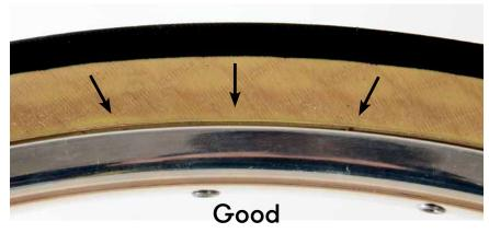
• If the line is even and parallel to the rim edge all around the tire (above, arrows), the tire is seated correctly. (Just below the molded line is a depression, which interlocks with the hook on the rim sidewall. This makes sure the tire remains seated correctly.)
