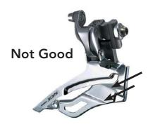
Front derailleurs for triples have steps in the cage (arrows) that must line up with the chainrings. With custom chainring combinations, they do not work well.
