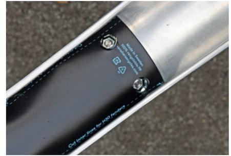
Now the mudflap fits over the 8 mm nuts for the fender eyebolts. To remove the mudflap, push up the center, starting at the fender end. Carefully pull the mudflap out of the fender edges.
