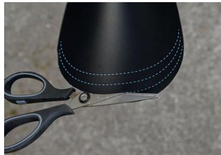
Tear off the top portion. Shorten the mudflap if the bottom edge is closer than 3-4 cm (1.5") to the ground. The width of the mudflap is designed for H-80 fenders.
