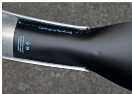
Insert the other edge of the mudflap into the rolled fender edge. Flatten the mudflap. If the mudflap cannot be flattened, it's too wide. Remove and trim.
