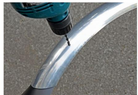
Drill the holes for the fender stay bolts through fender and mudflap. If your fender already has holes, redrill the holes (5 mm drill) through the mudflap.
