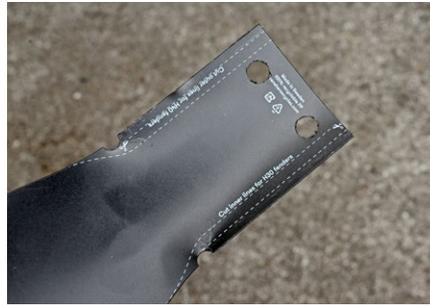
Optional: If you want to install and remove the mudflap without tools, remove the mudflap and drill out the holes in 0.5 mm steps until they measure 12 mm in diameter.
