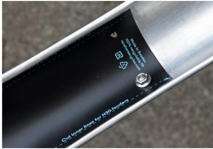
Install the fender eyebolts as you normally would. Pro Tip: If the mudflap doesn't reach the fender bolts, you can still use the mudflap. The cutouts at the fender corners will hold it in place.
