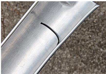
If you run a lighting wire through the rolled edge of the fender, use the top strip of the mudflap as a wire guide to trap the wire where it exits the fender edge and runs across the fender.
