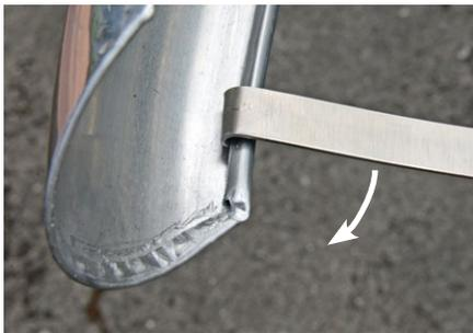
Remove the fender stays and bolts (if already installed). Open the rolled edge of the fender just enough to allow the mudflap to slide inside.
