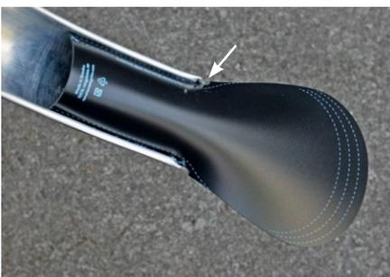
Insert the mudflap into one edge of the fender. Align the cutout with the crimped fender corner (arrow). Bend the center upward so it fits inside the fender.
