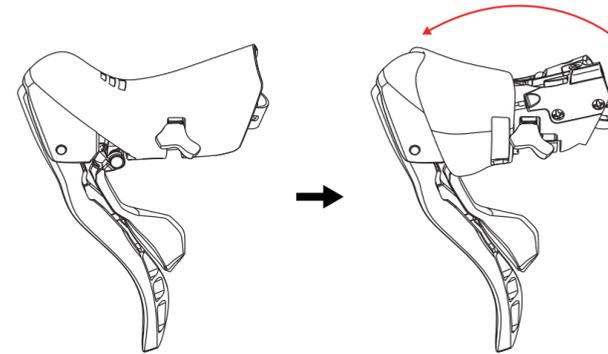
The clamp bolt is tightened at the factory, so please loosen it using a 4mm hex wrench before passing it through the handlebar.
