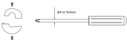
The cable pulleys are the same for both sides, but they will be installed with the opposite orientation. Please be sure to pay attention to the orientation when installing.
