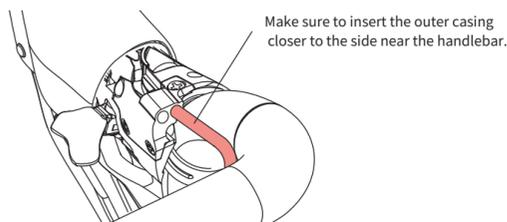
Make sure to insert the outer casing closer to the side near the handlebar.
