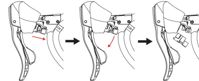
Install the under cover by following the removal steps in reverse order.
