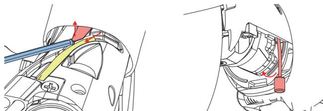
Fix the shift cable to the derailleur and confirm that the cable end is properly inserted before reattaching the under cover .
