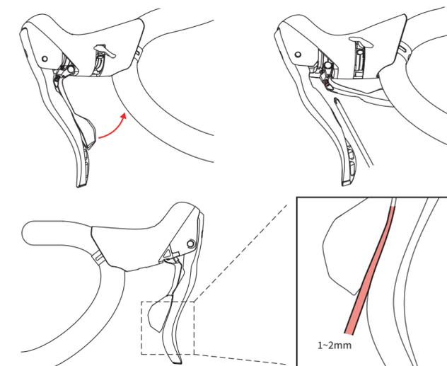
The gap between lever-A and the brake lever should be approximately 1 to 2 millimeters.
