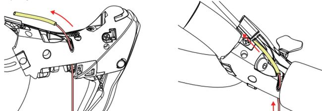
As shown in the diagram below, use a thin tool, such as a 2mm hex wrench, to lift the cable clip a few millimeters and fit the liner tube into the groove.
