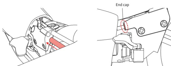
Thread the brake bead onto the brake cable and install it as shown in the diagram below.
