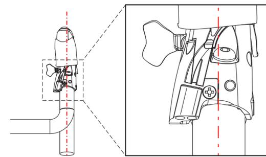
Tighten the clamp bolt using a 4mm hex wrench. (Maximum tightening torque 6Nm)
